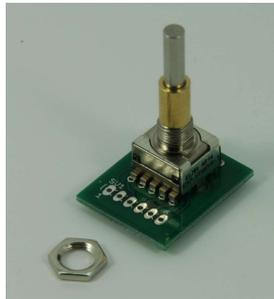
Figure 5 – (A1-1) Dual Concentric Rotary Encoder\*
